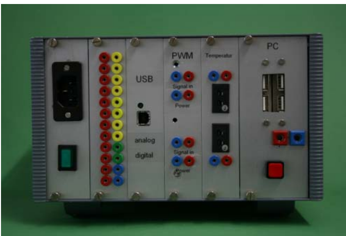
Fig. 2 Portable device for LabView applications with a mounted PC
