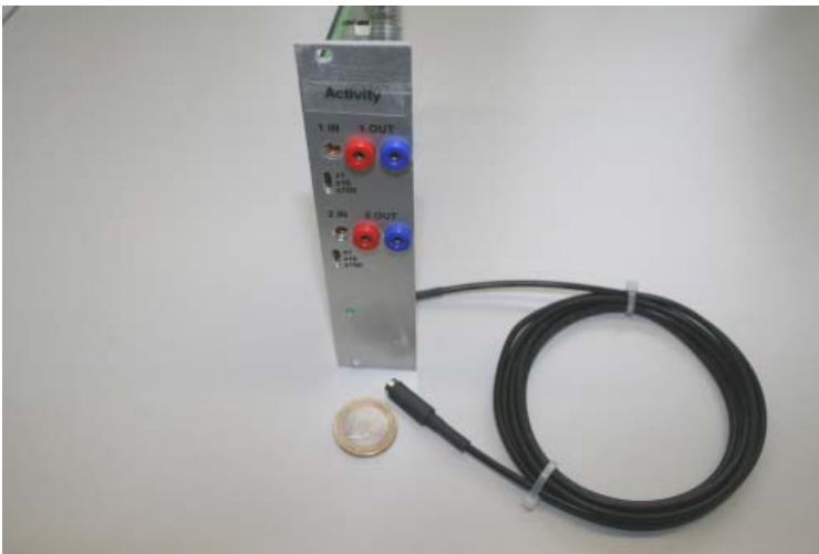
Fig. 3 Amplifier with photodiode radiation detector
